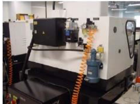
FIG(b): Pneumatic system of an automatic machine
